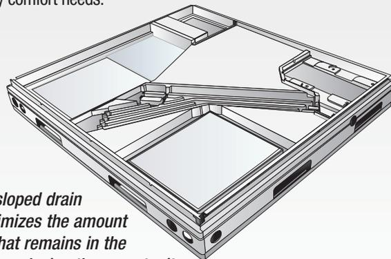
*The integrated sloped drain pan design minimizes the amount of condensate that remains in the indoor air cavity, reducing the opportunity for mold, mildew and odors to form.*
